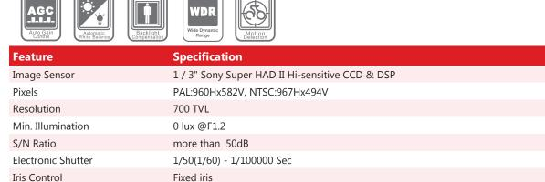
Lens 8mm Gamma Correction 0.45 White Balance (AWB) ON/OFF Selectable Gain Control (AGC) ON/OFF Selectable **Back Light Compensation** ON/OFF Selectable IR 72 LEDs, Upto 50 Mtrs
